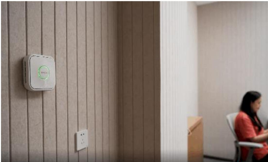
By continuously collecting quantity of real-time air quality data in various rooms of WELL Living Lab, Tongdy helps providing on-line and long-term data of air quality. The Well Living Lab can compare and analysis each air parameters including PM2.5, PM10, TVOC, CO2, O3, CO, Temperature and Relative Humidity, that was profound for Delos' future research in the field of green building and sustainable living health.
